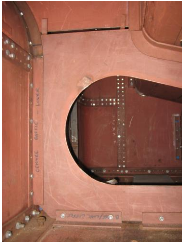
Parts of the upper and lower longitudinal baffles and their locating angles
