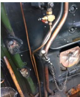
Two large copper injector feed pipes in cab £300
